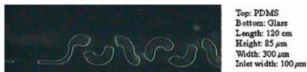
Figure 2. Segmented flow of gas bubbles and liquid slugs in the monochannel microreactor (Inlet part).
